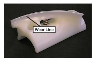
Figure 3-3 Auger Flight Wear
