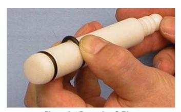
Figure 3-4 Removing O-Ring
