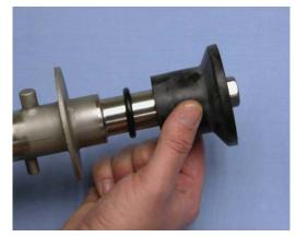
Figure 3-5 Rear Seal Assembly
