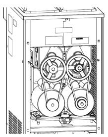
Figure 4-1 Belt Tension Adjustment
