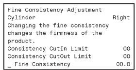
Figure 4-1 Fine Consistency Adjustment
