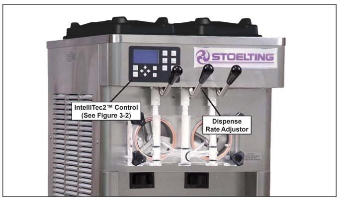
**Figure 3-1 Machine Controls**
