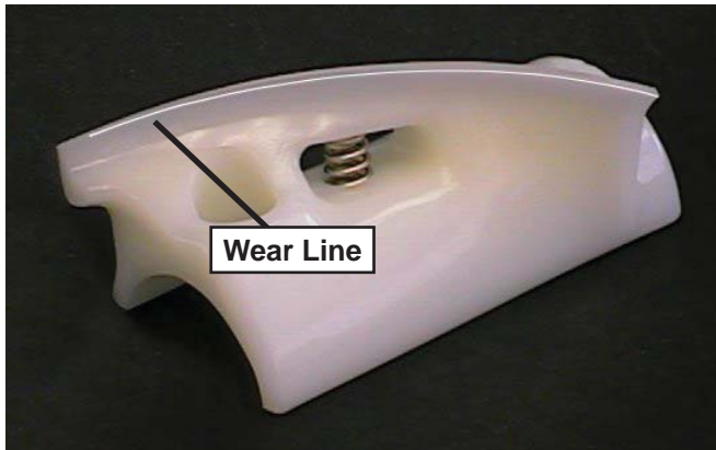
Figure 3-3 Auger Flight Wear
