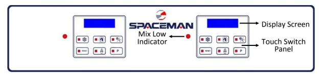
**MIX LOW INDICATOR:** A mix level indicating light is located at the front of the machine. When the light is "ON", it indicates that the mix hopper has a low supply of mix and should be refilled as soon as possible. Always maintain at least 2cm of mix in the hopper. If you neglect to add mix, a freeze-up may occur. This will cause eventual damage to the beater assembly, the dispensing door, and gear box.
