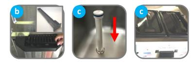
**IMPORTANT:** After sanitizing the machine, DO NOT rinse or touch areas that have been sanitized. Product must be added immediately. If new product will not be added immediately, rinse machine with clean water and loosen door hand-screws to allow cylinders to air-dry. Sanitize machine before using again.
